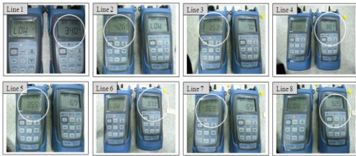
Figure 6. The optical power measured which pass through the optical splitter. The optical switch is controlled remotely by ACS
