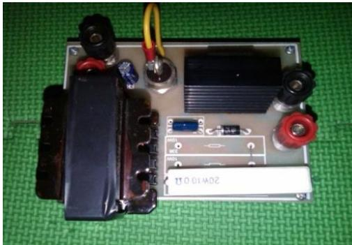
**Gambar 4.4 Hardware Buck Konverter I**
