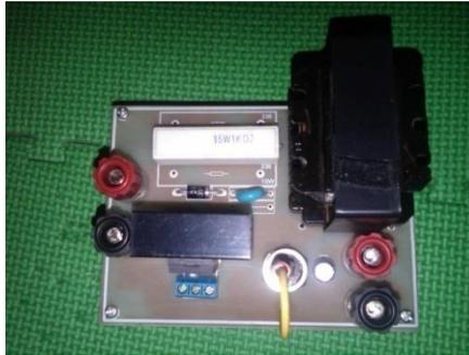
**Gambar 4.6 Hardware Buck Konverter II**
