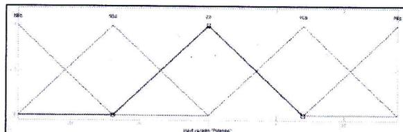
Figure 3: Membership function of steering system (potentiometer)
