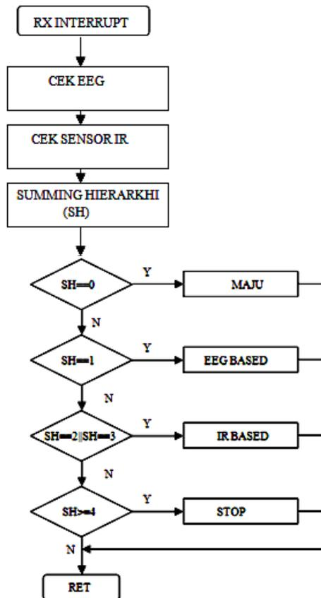
**Gambar 9.** Algoritma hierarki behaviour-based
