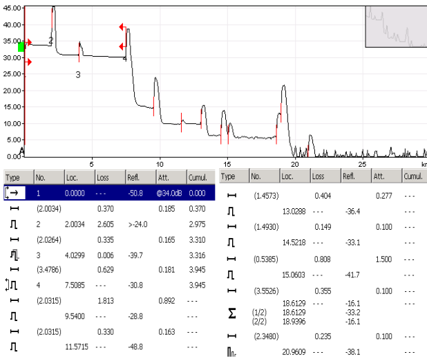
Figure 7. The network testing results for line 3 for the OTDR trace of downwardly testing in the proposed system architecture and the event table for OTDR trace
