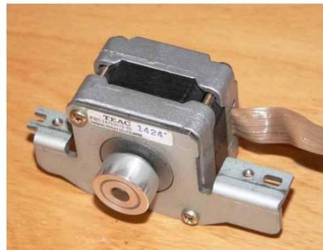
**Gambar 4:** Motor Stepper *Bipolar*
