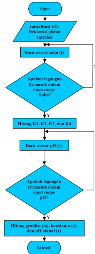
Gambar 2. Flowchart perancangan sistem sensor keasaman (pH)
