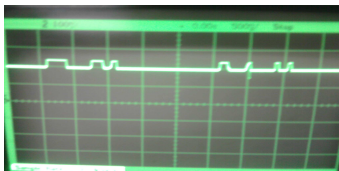
Gambar 4.3 hasil pengujian sensor rotary encoder
