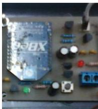
Gambar 2.7 *Layout* PCB Level Konverter X-BeePro
