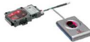
Gambar 6 Sensor Fingerprint U are U 4000B Digital Persona . [10]
